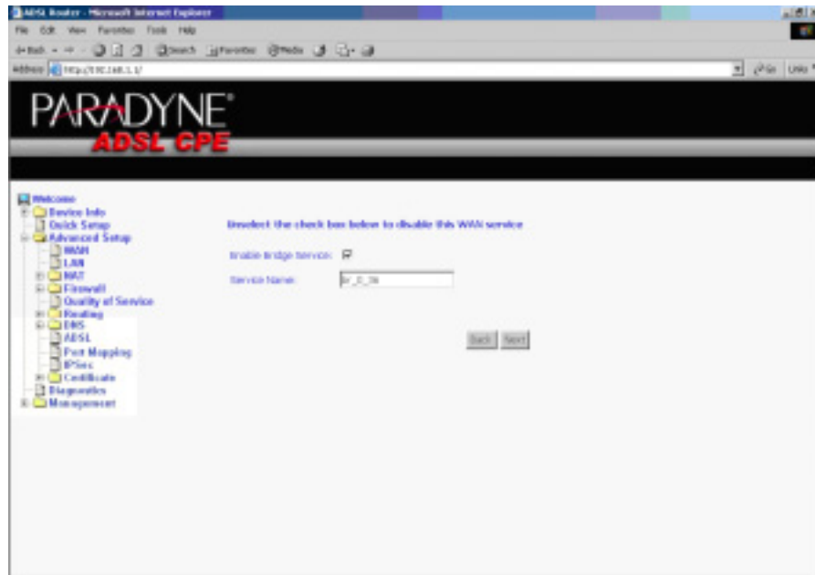
Figure 31: Enable Bridge Service
